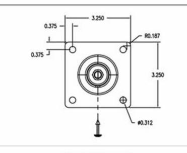
FLOOR CLIPPED LEG CHECK FLOOR PLAN FOR PROPER PLACEMENT OF UNIT. MARK LOCATION ON FLOOR. DRILL (DRILL BIT 204725-1) HOLE FOR TAPCON (204725). MOUNT MALE END (204629) TO FLOOR SLIDE LEG OVER FLOOR CLIP AND INSERT
