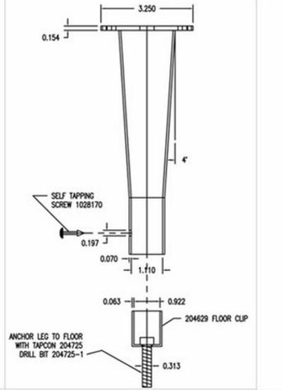
SCREW (1028170) TO HOLD UNIT IN PLACE.
