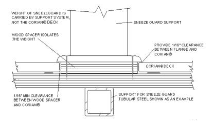
Figure 24 Sneeze Guard Assembly (one version)
