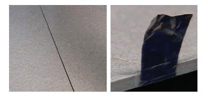
Figure 18 Hard Seaming and Seam Setting (Tape removed for detail)
