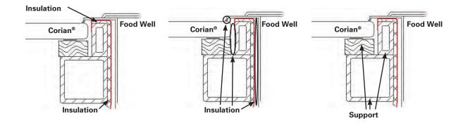
Figure 1 Insulate, Isolate, and Support Illustrations
