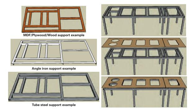
Figure 12 Acceptable Food Service Support Material Frames
