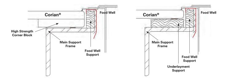
Figure 8A and B Cutout Cross Section with Angle Iron Support High-Strength Corner Block (left) and Underlayment (right)
