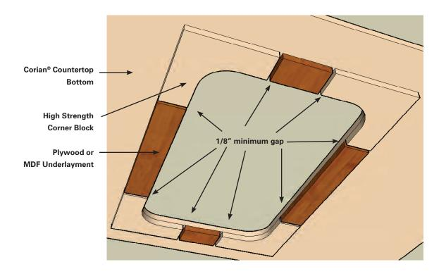
Figure 5 Cutout Perimeter Support Structure
